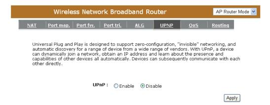
**Enable/Disable UPnP:** You can enable or Disable the UPnP feature here. After you enable the UPnP feature, all client systems that support UPnP, like Windows XP, can discover this router automatically and access the Internet through this router without having to configure anything. The NAT Traversal function provided by UPnP can let applications that support UPnP connect to the internet without having to configure the virtual server sections.
