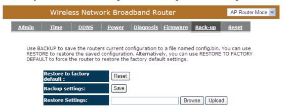
**Backup Settings:** This can save the Broadband router current configuration to a file named "config.bin" on your PC. You can also use the **Upload** button to restore the saved configuration to the Broadband router. Alternatively, you can use the "Restore to Factory Defaults" tool to force the Broadband router to perform a power reset and restore the original factory settings.
