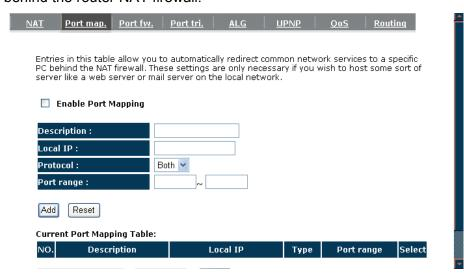
**Enable Port Mapping:** Enable or disable port mapping function.
