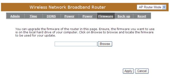
Once you've selected the new firmware file, click **Apply** at the bottom of the screen to start the upgrade process
