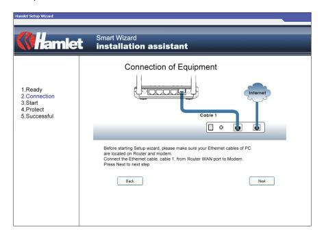
Check the MODEM and HNW300AP connection. It should be as shown below.
