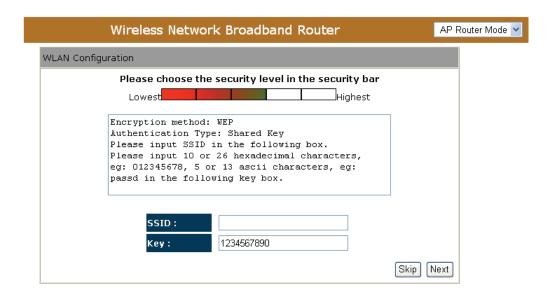
Enter the name for your wireless network (SSID) and security key
