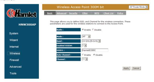
**Radio:** You can turn on/off wireless radio. If wireless Radio is off, you cannot associate with AP through wireless.
