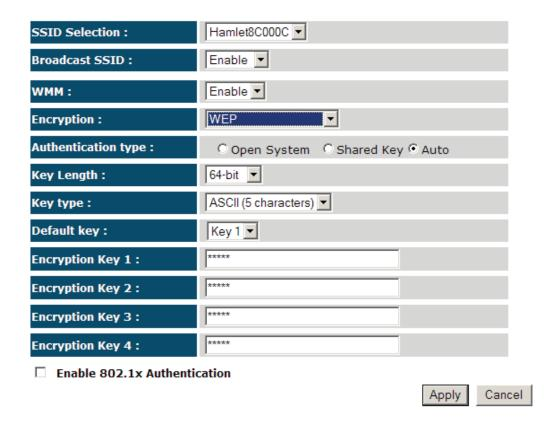
**Authentication Type:** There are two authentication types: "Open System" and "Shared Key". When you select "Open System", wireless stations can associate with this wireless router without WEP encryption. When you select "Shared Key", you should also setup a WEP key in the "Encryption" page. After this has been done, make sure the wireless clients that you want to connect to the device are also setup with the same encryption key.
