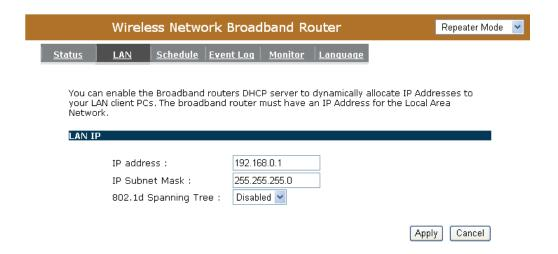
**IP address:** It is the router's LAN IP address (Your LAN clients default gateway IP address). It can be changed based on your own choice.
