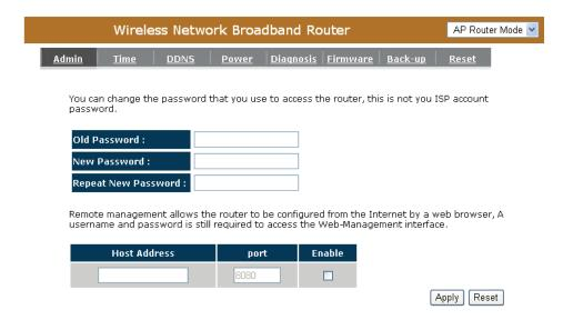
**Current Password:** Fill in the current password to allow changing to a new password.
