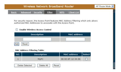
Enable Wireless Access Control: Enable the wireless access control function
