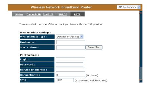
PPTP allows the secure connection over the Internet by simply dialing in a local point provided by your ISP provider. The following screen allows client PCs to establish a normal PPTP session and provides hassle-free configuration of the PPTP client on each client PC.
