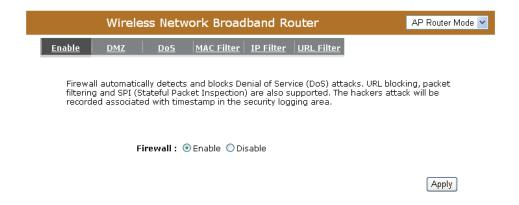
Note: To enable the Firewall settings select Enable and click Apply
