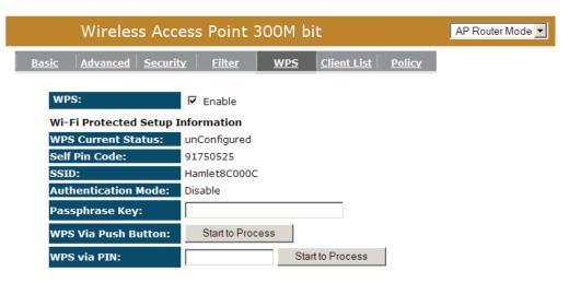
**WPS:** Check the box to enable WPS function and uncheck it to disable the WPS function.
