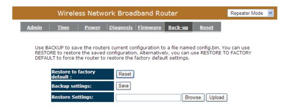
Restore Settings: This can save the Broadband router current configuration to a file named "config.bin" on your PC. You can also use the <Upload> button to restore the saved configuration to the Broadband router. Alternatively, you can use the "Restore to Factory Defaults" to force the Broadband router to perform a power reset and restore the original factory settings.
