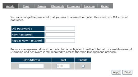
**Current Password:** Fill in the current password to allow changing to a new password.
