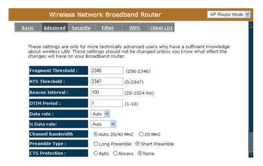
**Fragment Threshold:** This specifies the maximum size of a packet during the fragmentation of data to be transmitted. If you set this value too low, it will result in bad performance.
