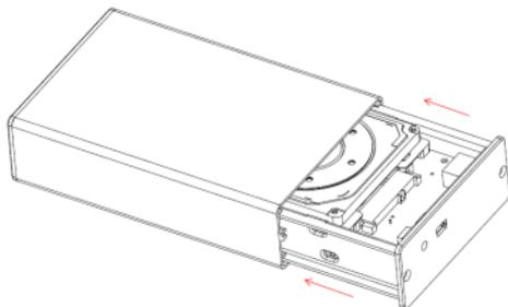
5. Close the rear cover. The HDDs installation is now completed.
