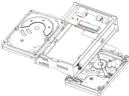
4. Insert the inner HDD tray back into the aluminum housing.
