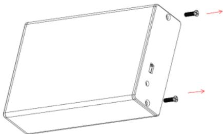
2. Pull out the inner HDD tray from the aluminum shell.
