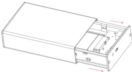
3. Insert the HDDs into the 7+15P SATA connectors on the corresponding PCBA. Fix the HDDs by HDD buckle.
