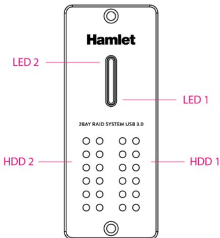
If one drive fails and the RAID mode is set to RAID0 or JBOD, the data will be lost and the system can not be accessed again until the drive have been replace.
