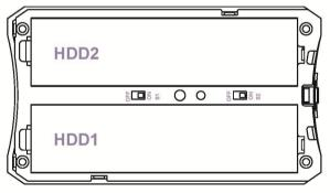
S1/S2=ON/ON, Normal Mode S1/S2=ON/OFF, JBOD Mode S1/S2=OFF/ON, RAID-0 Mode S1/S2=OFF/OFF, RAID-1 Mode
