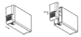
Install the hard drives as illustrated below with the top of the drives, where the label is located, facing each other. Push the drives lightly into place.
