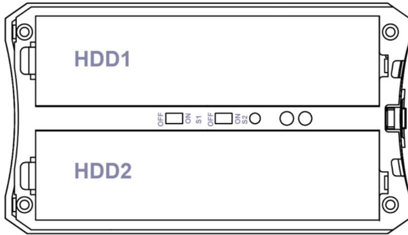
If one drive fails and the RAID mode is set to RAID0 or JBOD, the data will be lost and the system can not be accessed again until the drive have been replaced.
