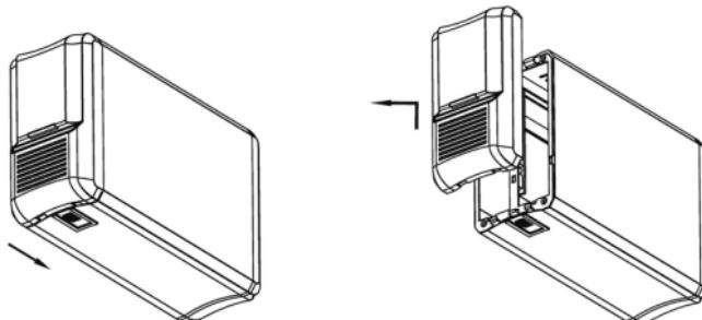
2. Install the hard drives as illustrated below with the top of the drives, where the label is located, facing each other. Push the drives lightly into place.
