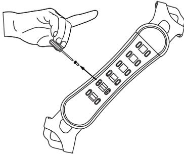
1. Use the screwdriver provided to release the two locking screws of the frame.
